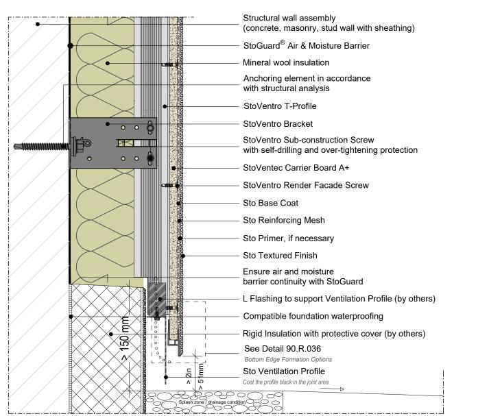
If the StoVentec Carrier Board projects into the splash zone when it is installed, provide the system with additional protection against moisture penetration and ensure constant system ventilation by taking structural and maintenance measures. Constant, excessive stress from moisture can damage the system. The planner must determine the height and position of the splash zone on a project-specific basis.
